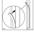
From the plastic cover (E), which is used to cover the hinge with the pivot pin, you must take away the part as indicated in the drawing.
